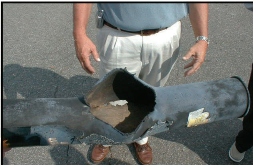
Plastic reloadable tube that experienced severe blowout and warping when shell exploded upside down inside the launcher tube.
